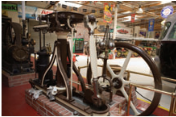
This 1831 steam engine is fully functional with its lower sleeve replacement — the brass part suspending the spherical flyweights. The engine is one of two stationary engines Jay Leno houses at Big Dog Garage.
