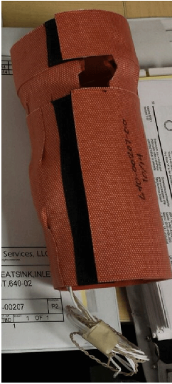
The finished vulcanized rubber shell manufactured with a mold produced using a 3D Systems sPro 60 SLS system.
