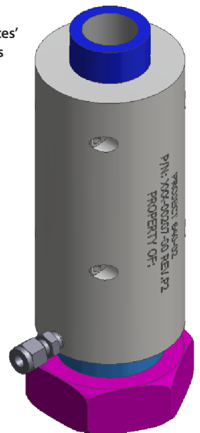
A CAD model of the assembly around which Cooper Environmental Systems created a 3D-printed mold for a fitted vulcanized rubber shell.
