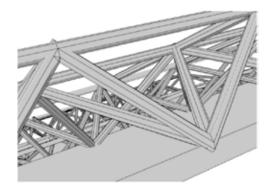
These materials can provide good energy absorption characteristics and good thermal and acoustic insulation properties as well. Cellular materials include foams, honeycombs, lattices, and similar constructions.
