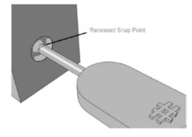
Note in the above stick, to "tag" connector the junction between the stick and the part is in a depressed filleted pocket, this reduces the impact on the mechanical integrity of the part. Also note the snap point in this case, a V notch modeled into the stick. The same can be applied to chains where you want to enable easy controlled removal of the tag.
