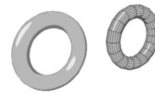
Invest time in getting a single link optimized before array duplication. Consider using a polygon instead of the circle to speed up link duplication and manipulation in CAD.
