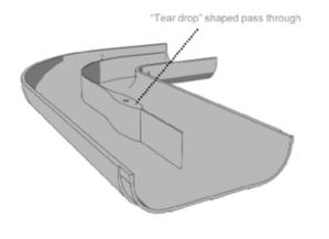
Always apply generous fillets to baffles to prevent side walls of ducts from splitting, especially if component will be exposed to pressure and/or cycling of temperature.
