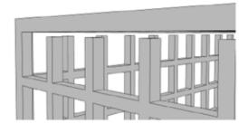
In applications requiring additional post processing, such as sterilization for surgical use, the batch can transition through the various processes within the cage. To remove the parts consider CAD modeling in hinge doors, apply snap-off regions or, as in this example, connect the lid with the four corner posts that can be cut off with wire snips.
