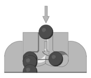
Once all the bearings have been dropped into the chase, a plug can be fixed to seal in the chase.
