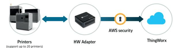
Data is collected from the printer(s) by the adapter, converted to an internal representation, and securely transmitted to an Amazon Web Services (AWS) hosted instance of the Thingworx platform (from PTC). 3D Systems controls and administers the Thingworx server. Only authorized 3D Systems employees have access to the AWS server.
