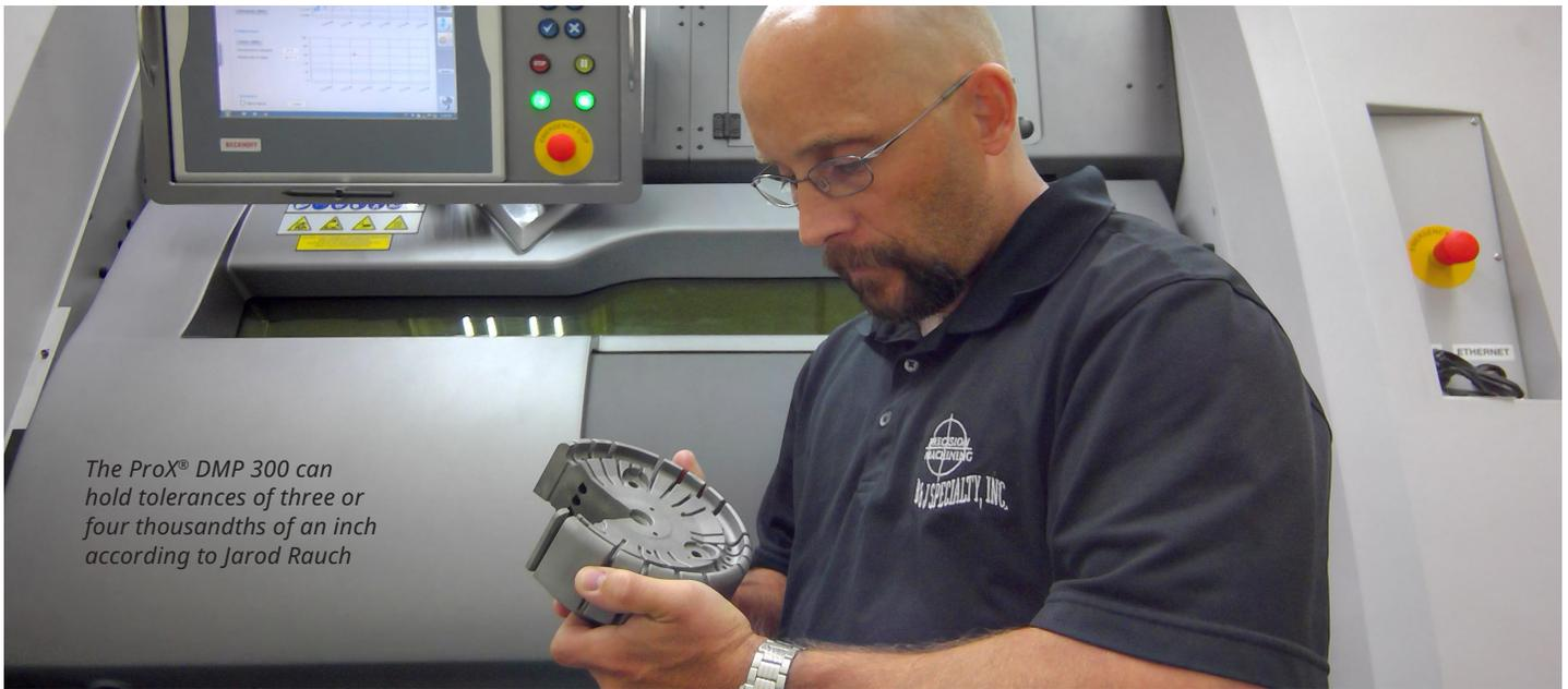
*The ProX® DMP 300 can hold tolerances of three or four thousandths of an inch according to Jarod Rauch*
