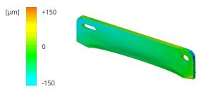
**High accuracy** after support removal and sandblasting as measured by a 3D scan.
