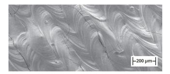
DMP Flex 350 allows **fully molten tungsten** material. Additively manufactured pure tungsten does contain micro cracks and is brittle, limiting its use for mechanically loaded components.
