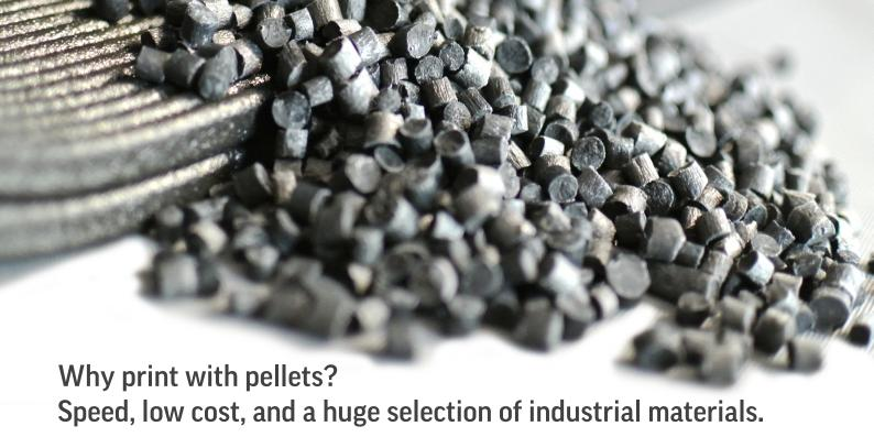
As the raw form of most thermoplastics, pellets are the lowest cost feedstock available for additive manufacturing, and they're available in hundreds of formulations.
